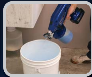
3. Reverse the tip and flush.
